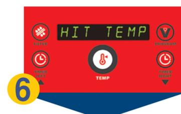
**6** Once the oil level has been checked and verified, press the TEMP button. The burners will automatically turn back on and the fryer will resume heating. **HIT TEMP** displays.
