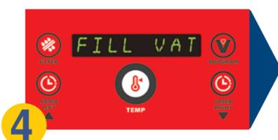
**4** When filtering is finished, close the red drain valve by turning the red drain handle. **FILL VAT** displays.
