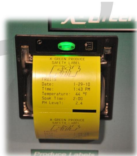
Figure 4: The X-Green label printer gives operators and customers complete information about the wash cycle of the produce.
